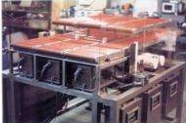
This is a three lane system, each with its individual Weigh-Cells, Setpoint Controllers, Input Conveyors, Scale Conveyors, Output Conveyors, and Sorting Conveyors. Sorting took place at 30 packs of lunchmeat per minute per lane. That is 90 packs of lunchmeat per minute total!
