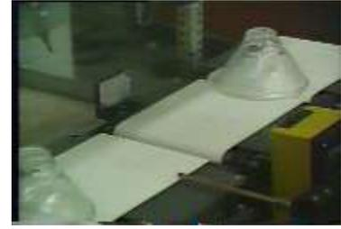
This system is designed to sort the over/under glass spot-light backs, out of the process at a rate approaching 40 parts per minute. This system is designed for parts 500 grams and less in weight, with an accuracy of  $\pm 0.02\%$ .
