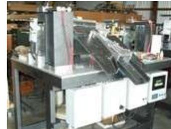
This system is designed using walking-beam technology to sort the over-weight and under-weight billets out of the process at a rate approaching 40 parts per minute. This system is designed for billets 10 kgs and less in weight, with an accuracy of  $\pm 0.02\%$  with a 10 kg part.
