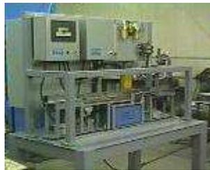
This system is designed to sort the over-weight and under-weight billets out of the process at a rate approaching 60 parts per minute. This system is designed for billets 500 grams and less in weight, with an accuracy of  $\pm 0.05\%$  for a 500 gram part.
